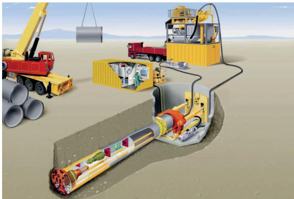
*Schema microtunneling (fonte: Herrenknecht)*
